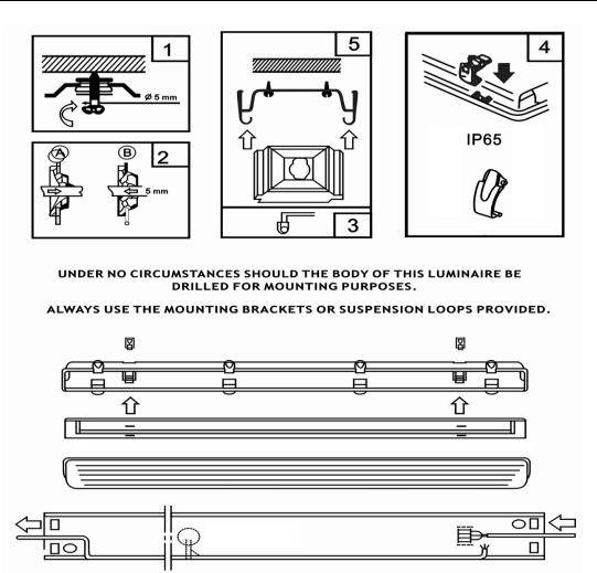
Please Note: Any additional power feed cable should be retained in such a way as to prevent contact with any control gear.
